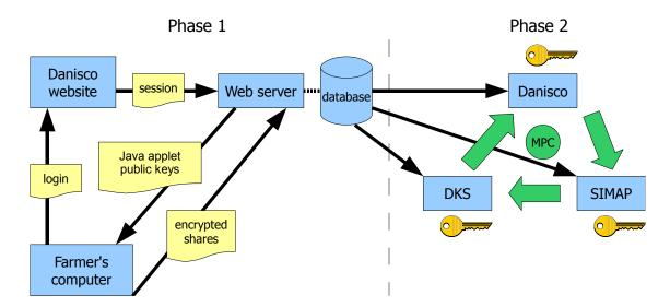
Figure 2: The architecture used in the Danisco auction.
