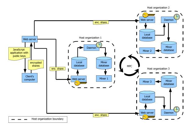
Figure 4: The proposed architecture using JavaScript technology and three shared public keys.
