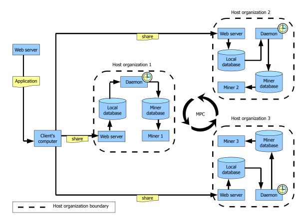
Figure 3: Data movement in the proposed architecture.
