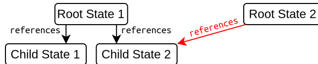
Figure 2: An enclave may need to split its state into multiple files. For example with a key-value store, the full set of small keys could be stored in the root state, and each large value could be stored in a separate file. The enclave code should ensure that a fresh or forked root state cannot successfully use an unrelated child state.
