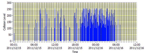
Figure 7: Collision reports from Estonian AtoN No. 861 due to short mooring pull during a buildup of north winds that started approximately at noon of 2011-12-15 and sustained speeds in gusts in excess of 12 m/s to 19 m/s. Wind speed dropped below 8 m/s and started to change the direction at 06:00 (UTC) the next day.
