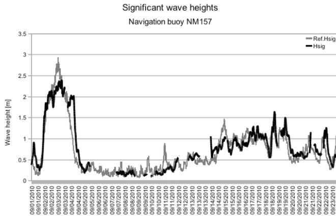
Figure 3.10: Results of the first test period on buoy NM157 (Sept. 2010) [69]
