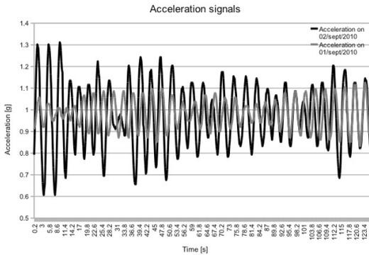
Figure 2: Acceleration signal packages recorded in stormy (02/sept/2010) and calm weather (01/sept/2010)
