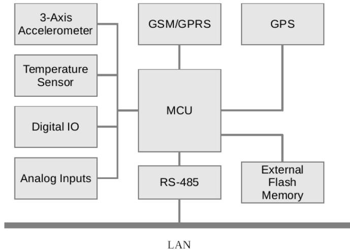
Figure 3.3: Telematics Module block diagram
