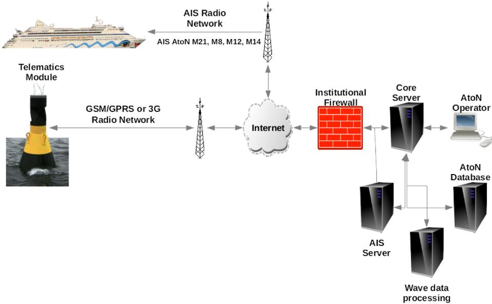
Figure 3.1: Typical synthetic AIS AtoN system setup
