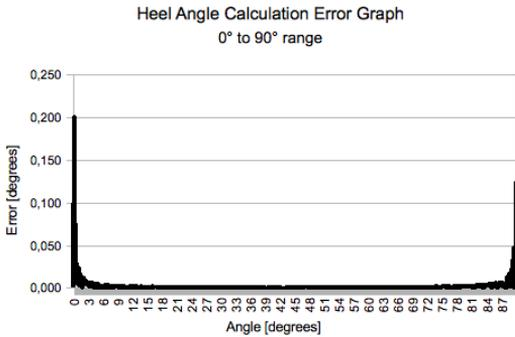
Figure 3: Heel angle calculation errors over the full range of 0° to 90°.
