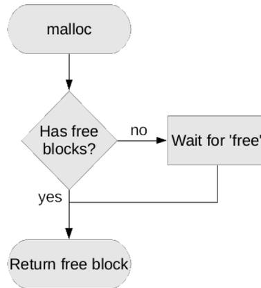
Figure 4.3: Pooled allocator
