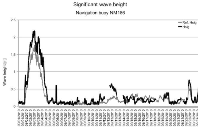
Figure 3.11: Results of the first test period on buoy NM186 (Sept. 2010) [69]
