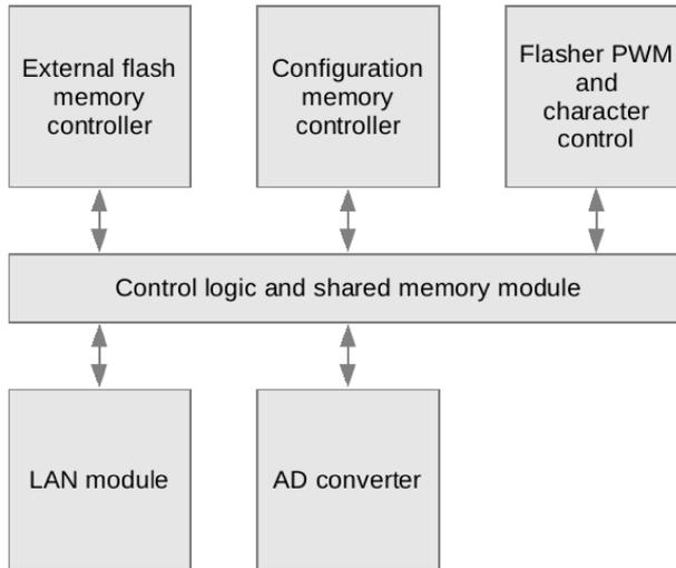
Figure 3.5: Flasher internal software modules
