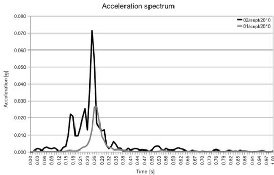
Figure 3: Acceleration spectrums calculated from data of stormy (02/sept/2010) and calm weather (01/sept/2010)
