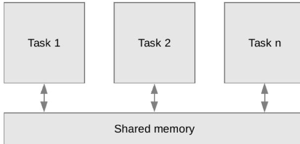
Figure 3.4: Communication between tasks by using shared memory
