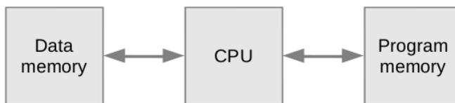
Figure 2.2: Harvard architecture in programmer's view
