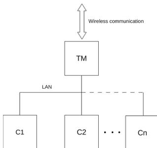
Figure 1: AtoN internal network
