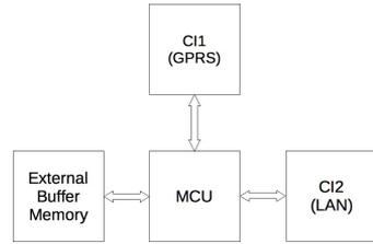
Figure 2: Telematics module
