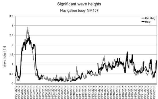
Figure 5: Results of first test period on buoy NM157 (Sept. 2010)
