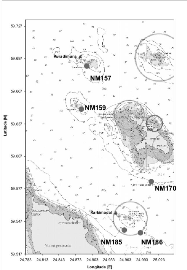
*Figure 3.9: Location of navigational buoys hosting the acceleration sensors used in the wave parameter measurement experiment, and pressure based wave measurement equipment used for reference measurements shown with triangles [69].*
