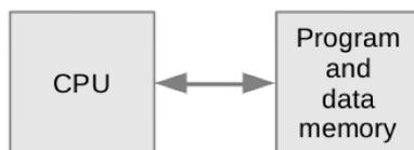
Figure 2.3: von Neumann architecture in programmer's view
