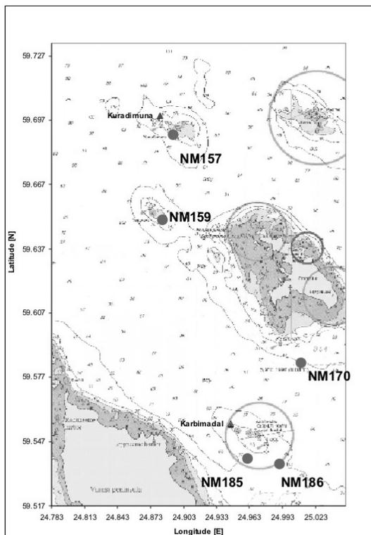
Figure 4: Location of navigational buoys hosting the acceleration sensors used in the wave parameter measurement experiment, and pressure based wave measurement equipment used for reference measurements shown with triangles.
